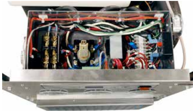
Typical Electrical Panel : 3/4 ton units
