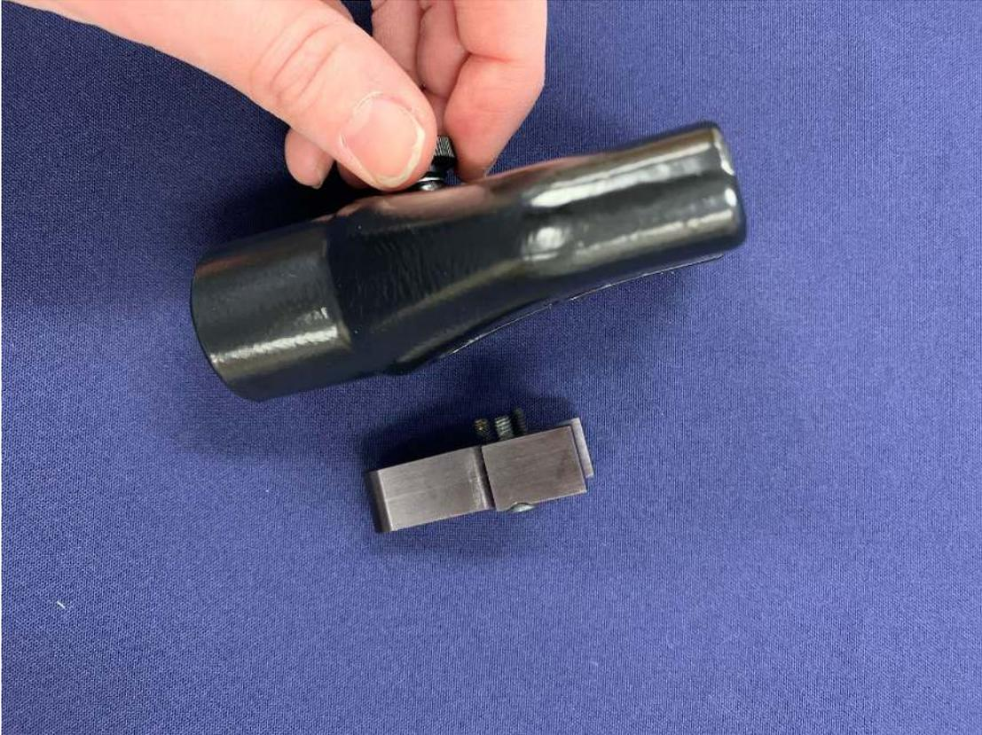
5. Install the adapter bracket to the 810 vacuum adapter with the screws provided.
