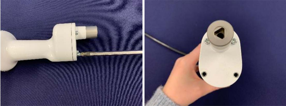
3. Attach the BD022 Vacuum Adapter to the saw using the long screws provided.
