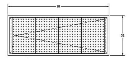
**Frame:** Material on the cart frame is 1-1/2" heavy gauge wall stainless steel tubing. All welding is continuous with an approximate 1/8" radius bead. All welds are clean and free of burrs and discoloration.
