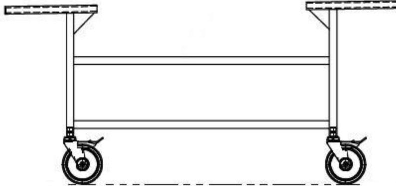
**Casters:** Heavy-duty 8" diameter casters are provided with three wheel brakes and one swivel lock.
