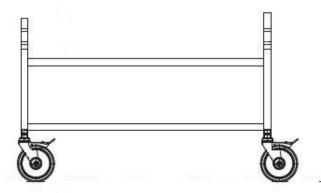
**Welding:** All welding is TIG type welding utilizing only stainless steel as a filler media. All weld fillets are approximately 1/4" (.64 cm) diameter. All welds are brushed clean removing any weld burns and burrs.
