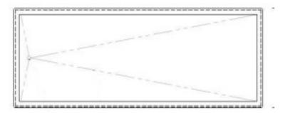
**Removable Cart Top: GA300** Fabricated of 14 gauge 304 stainless steel with #4 satin finish. The top is elevated with a trough around the body platform and dimpled toward the drain hole. A drain plug on a chain is provided. All exposed welds are ground smooth and grained to match a #4 satin finish. Top dimensions are 80.5" x 32"
