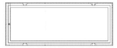
**Removable Cart Top: GA800** Heavy-Duty Blue Vacuum Formed construction with inner drain trough. Includes Plug and Chain. Top Dimensions are 82.10" x 32.25"
